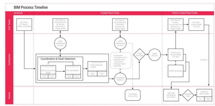
BIM Execution Plan During Design-to-Engineering-to-Construction Process
